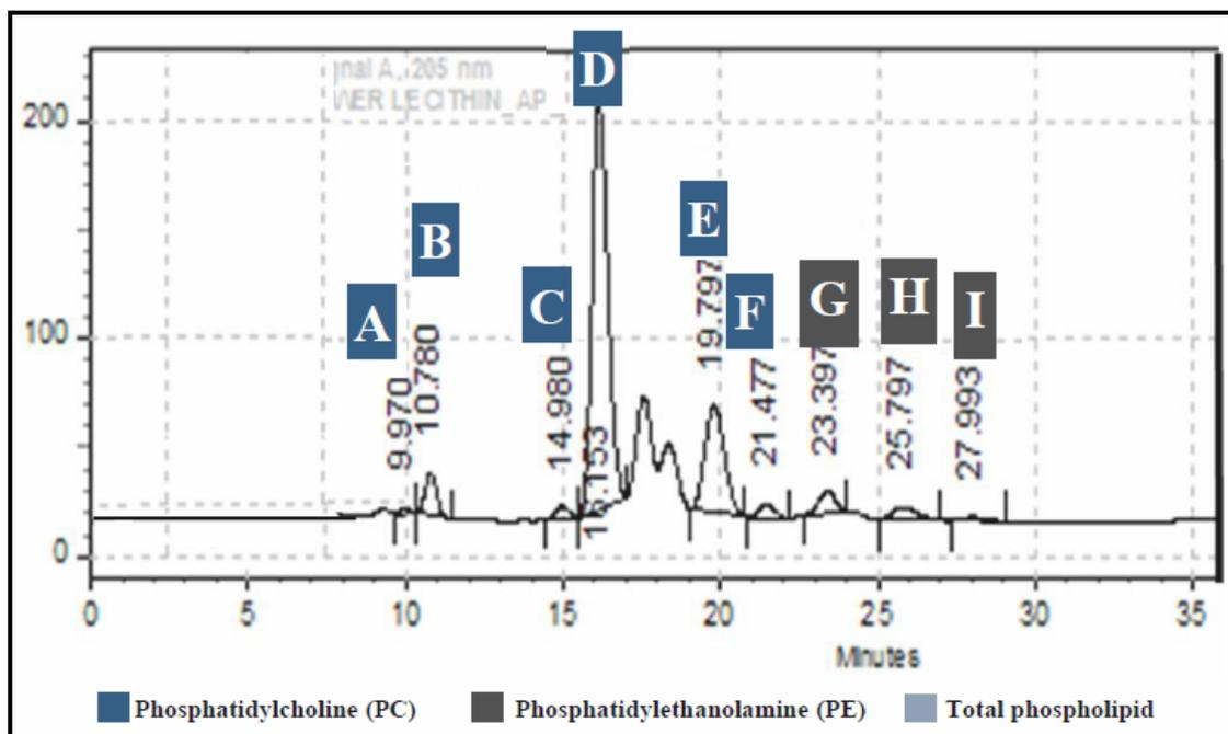
Figure 3: Chromatogram of Liposome with peaks of PC and PE
