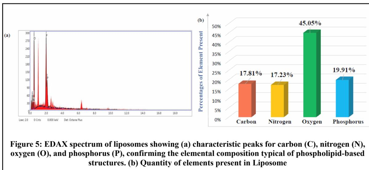
**Figure 5: EDAX spectrum of liposomes showing (a) characteristic peaks for carbon (C), nitrogen (N), oxygen (O), and phosphorus (P), confirming the elemental composition typical of phospholipid-based structures. (b) Quantity of elements present in Liposome**
