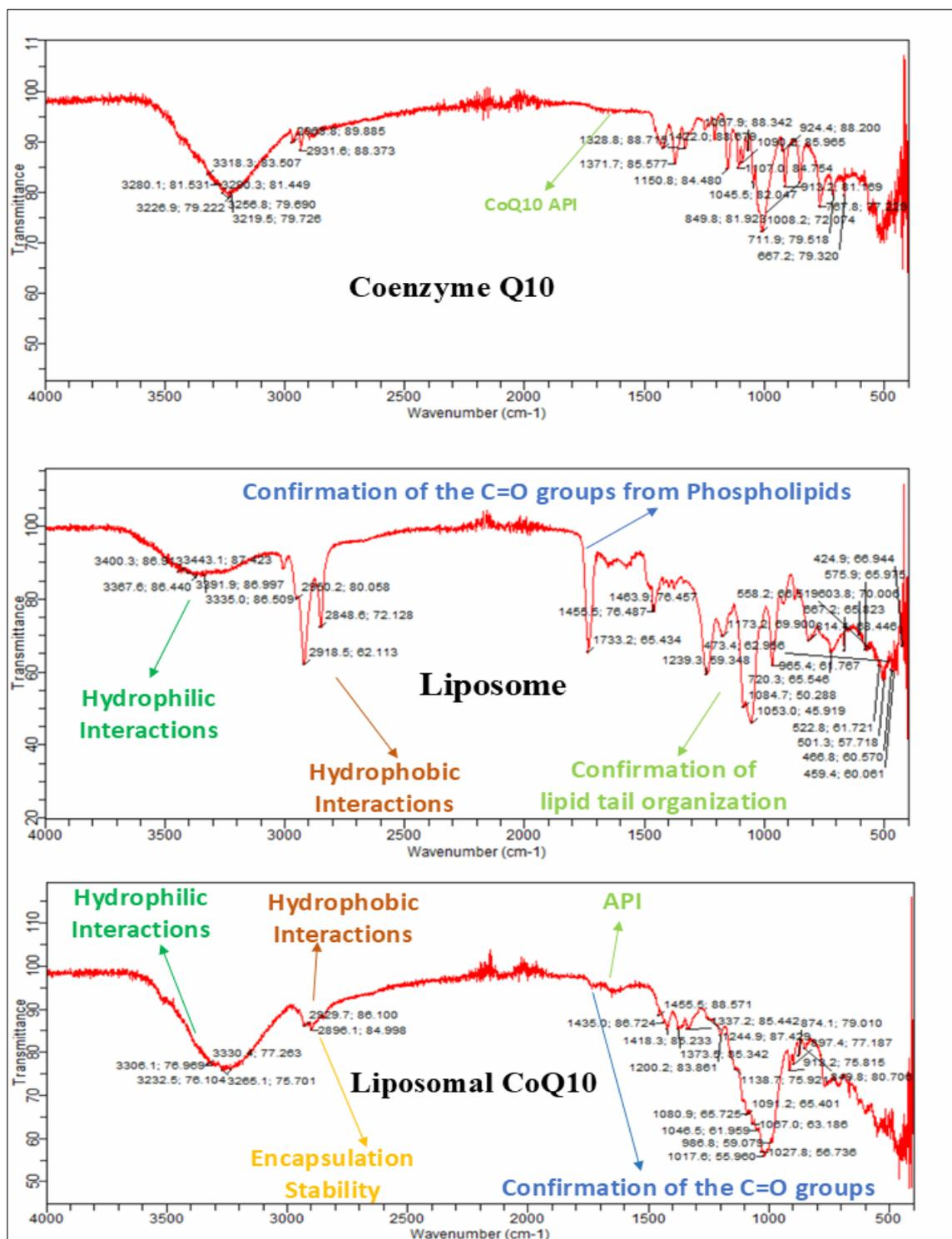
Figure 10: FTIR Transmission spectrum showing bands at different wavelengths of (a) CoQ10 API, (b) Liposome and (c) Liposomal CoQ10
