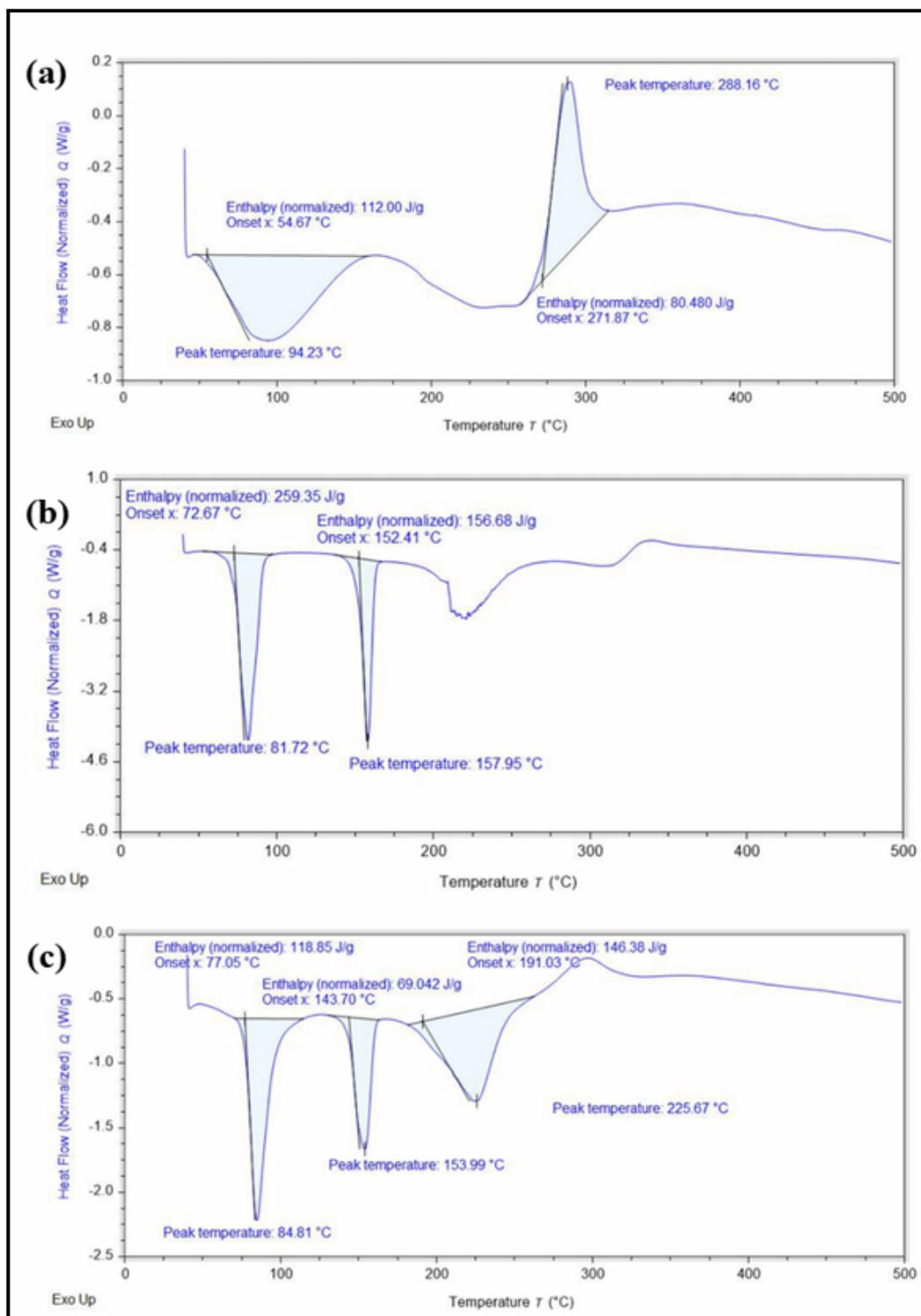
Figure 15: DSC Thermogram of (a) Liposome, (b) CoQ10 API, and (c) Liposomal CoQ10
