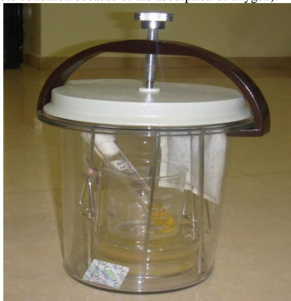
**Fig. 6: Anaerobic Chamber**
