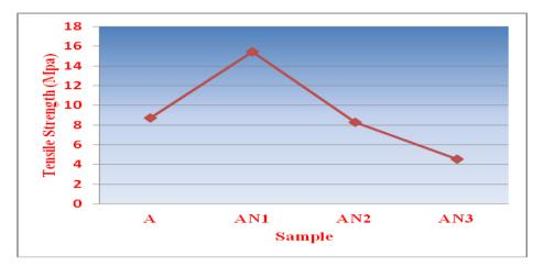
Figure 3: Variation in Mechanical strength with increasing filler loading
