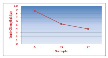
Figure 1: Variation in mechanical strength with varying ratio of starch and PVA in the blend
