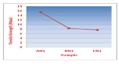
Figure 2: The Change in Mechanical strength in 1% clay filled sample of starch and PVA blend with varying blend ratio
