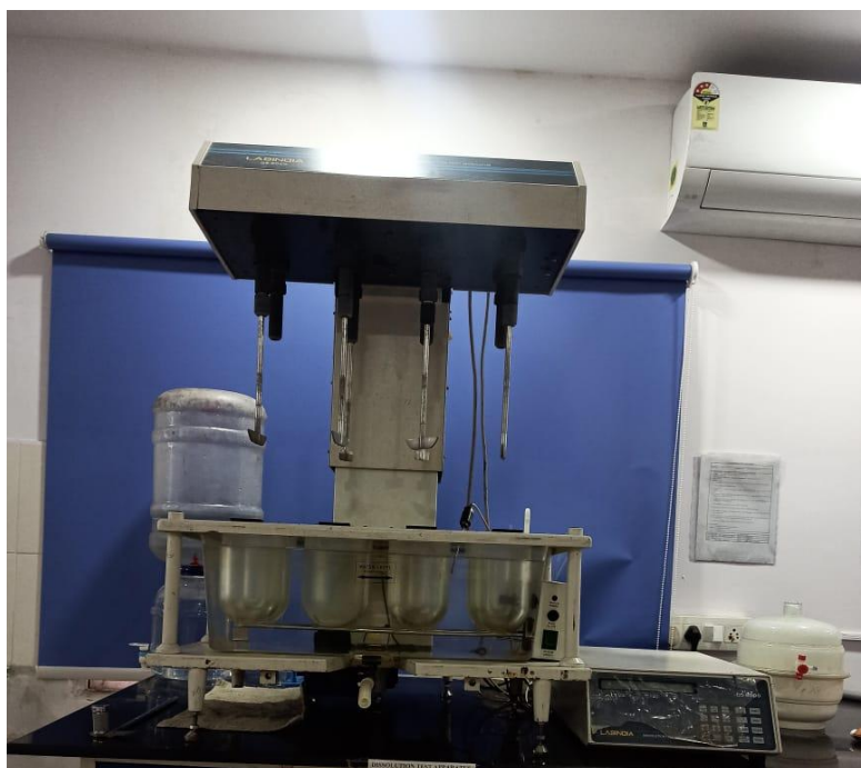
Fig 4 8 dissolution USP XIII Rotating basket apparatus
